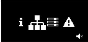
Whenever the crossed speaker symbol appears in the right corner of the main menu, the device's sound is globally switched off. If there is no speaker symbol displayed, the sound is globally switched on.
