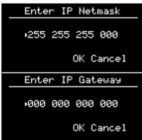
Enter the IP gateway. In normal cases this can be left unchanged to 0.0.0.0.
