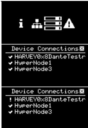
With the menu entry “Device Connections” highlighted push the rotary knob to enter the entry.
