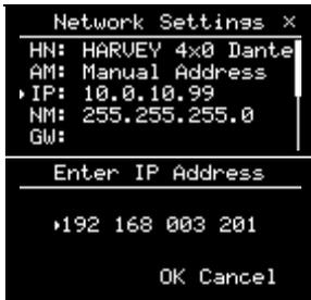
By entering the “IP Address” entry, when the device is set to “Manual Address” in our example, ...
