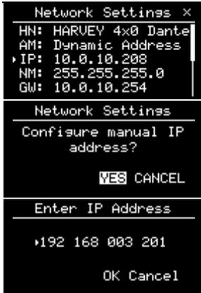
By entering the “IP Address” entry, when the device is set to “Dynamic Address” in our example, ...
