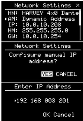
By entering the Address Mode entry, which is set to “Dynamic Address” in our example, ...
