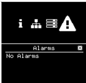
With the menu entry “Alarms” highlighted push the rotary knob to enter the entry.
