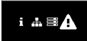
Main menu with menu entry "Alarms" highlighted. This entry informs about current errors of the device. See section 4.2.4
