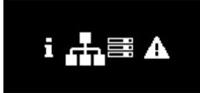
Main menu with menu entry "Network Settings" highlighted. See section 4.2.2 for further information on the "Network Settings". This entry is useful to change the device's network settings.
