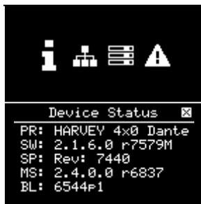
With the menu entry "Device Status" highlighted push the rotary knob to enter the entry.
