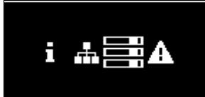
Main menu with menu entry "Device Connections" of Hypermatrix devices highlighted. This entry informs about the current inter-device network connection status of Hypermatrix devices. See section 4.2.3
