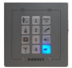
Blue: RC12 has network link and waits for pairing with a HARVEY Pro device.
