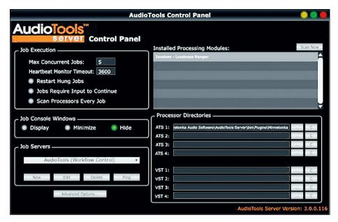
ISOSTEM Loudness Ranger comes as a plug-in of the Minnetonka Audio Tools Server 3. It is delivered with the version 3.0 installer of Minnetonka ATS. In this low level computation environment, it performs a 2-hours program in less than 4 minutes with an i7 32Go RAM standard PC.
